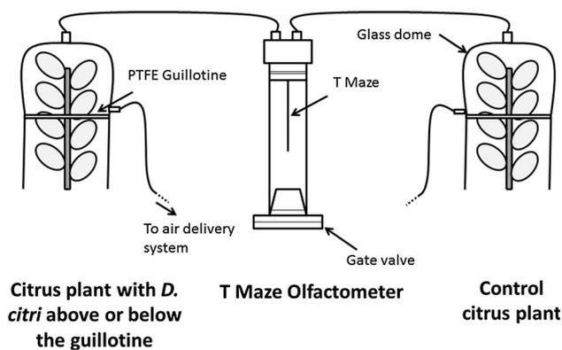
**Fig. 1** Schematic diagram of the olfactometer apparatus used to test the effect of *D. citri* feeding on behavioral response of *D. citri*
