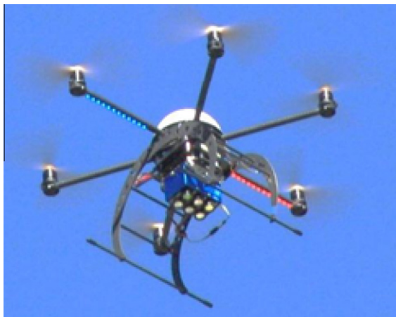
Fig. 1. UAV with multiband sensor used for data acquisition from citrus orchard.
