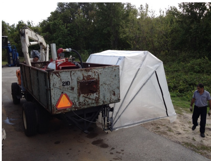
Figure 4: The CREC prototype steaming system mounted to a converted citrus hauler (goat)
