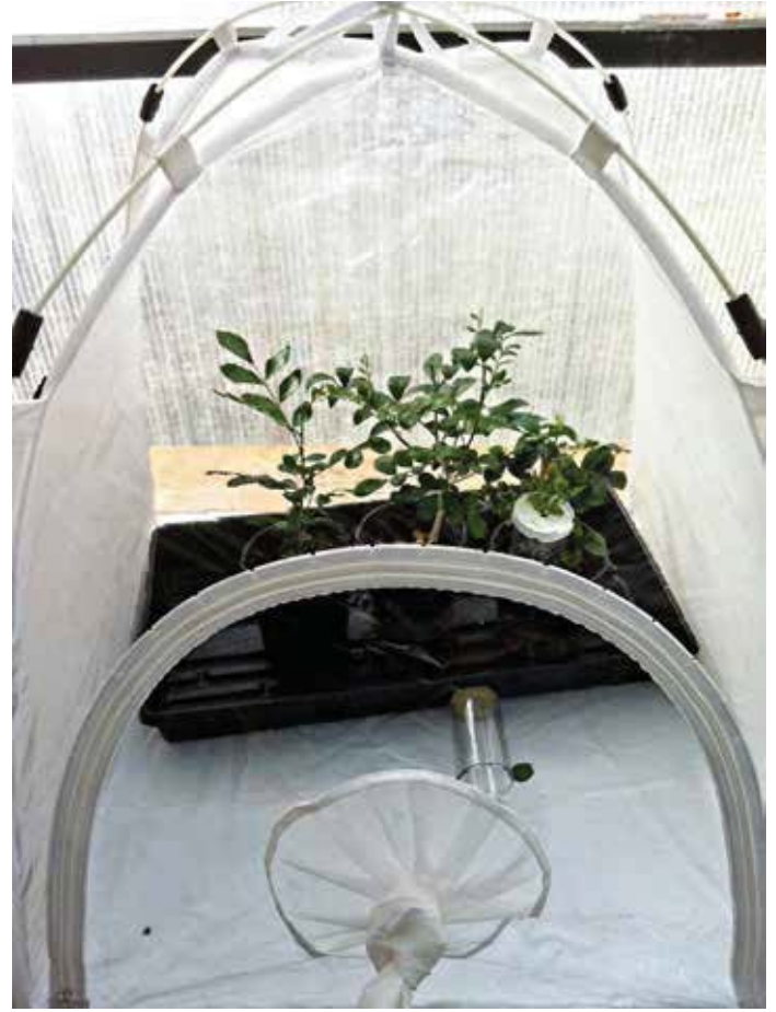
Photo 4. Plastic cage with a cloth sleeve and a zippered front for addition and removal of plants and insects. This cage is called a BugDorm.
