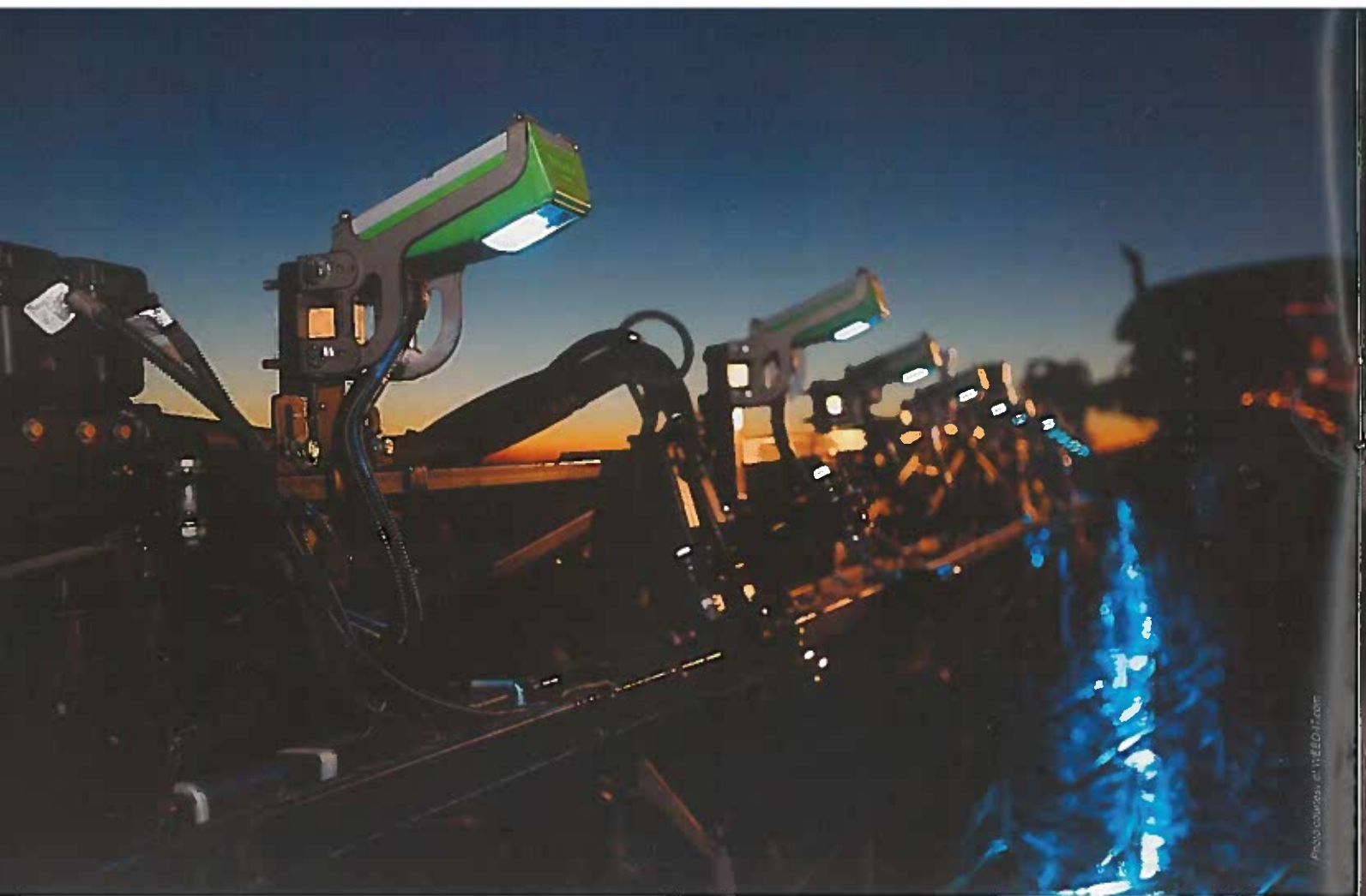
Figure 1. WEED-IT's precision spraying system utilizes blue LED lighting to identify weeds for spot spraying.
