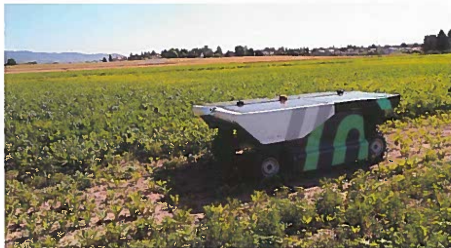
Figure 4. AVO is a solar-powered autonomous weeding robot.
