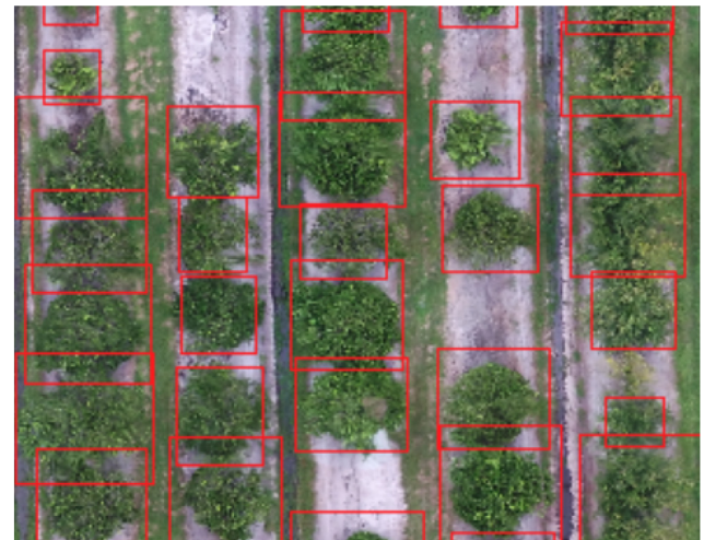
Fig. 7. Example of Faster R-CNN tree detection on part of Grove A.
