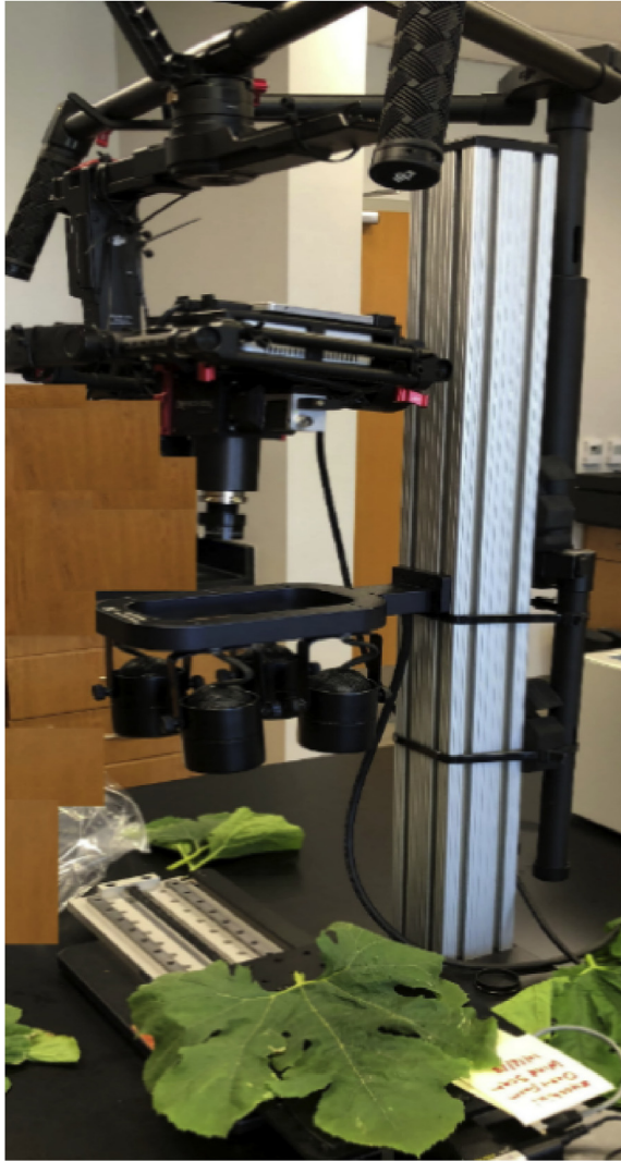
Fig. 2 – Laboratory spectral measurements of squash leaves using a benchtop hyperspectral imaging system.
