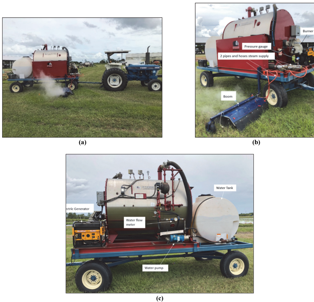
Figure 2. (a) side view of the weed steamer. Main components of the weed steamer: (b) right side view (includes the boom section, pressure gauge, pipes etc.); (c) left side view (includes the water tank, water pump, and electric generator).
