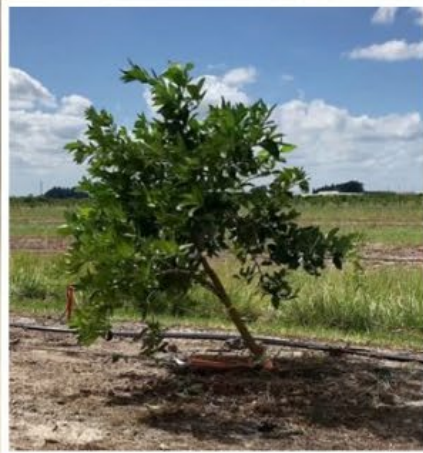
The study simulated wind-induced uprooting by pulling trees over with an electric truck winch. The maximum pulling force was measured using a digital force gauge.
