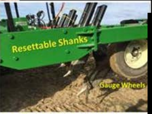
An Integrated System: "State of the Art" Tracking, Fumigating & Bedding Machine
