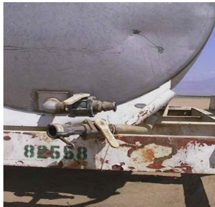
Unsecured Discharge Valve
