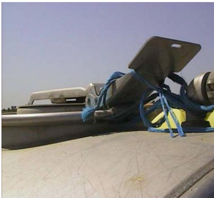
Improper Tank Security
