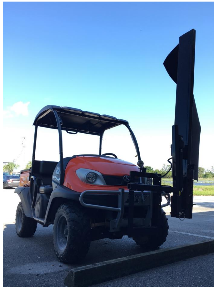
Figure 2. Citrus Herbicide Boom with Compressed Carbon Dioxide Sprayer Mounted on an ATV
