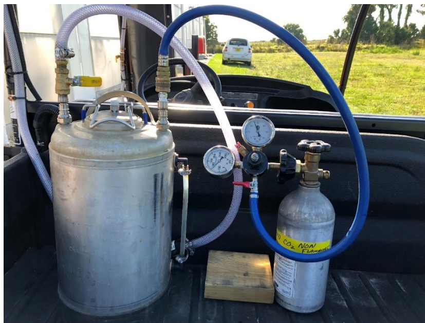
Figure 1 Liquid Carbon Dioxide and Spray Tank Assembly
