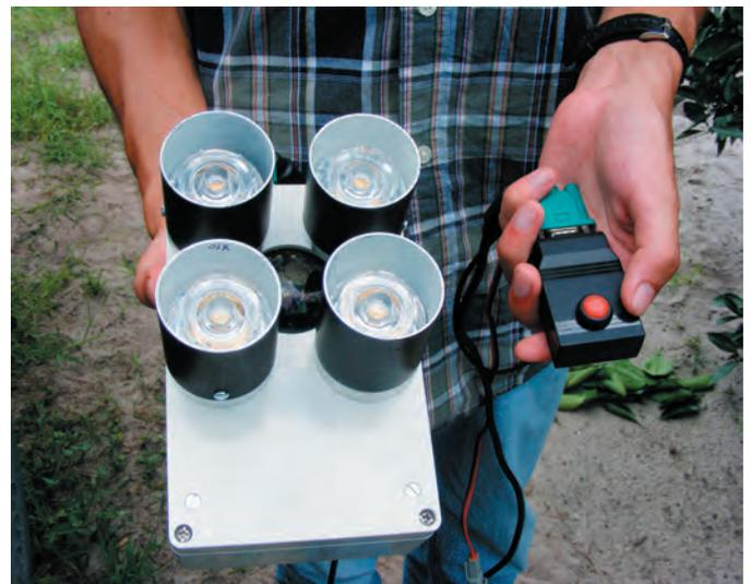
Fig. 3. Multi-band active optical sensor.
