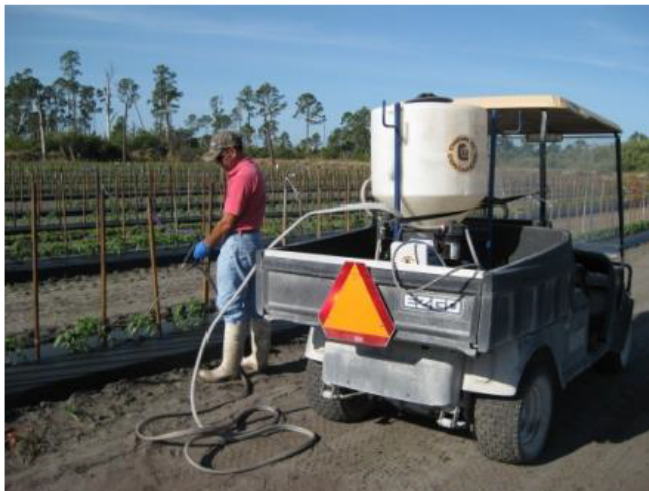
Figure 1. EZ-Dose® sprayer 45 PSI delivering 3.7 gpm for drench application
