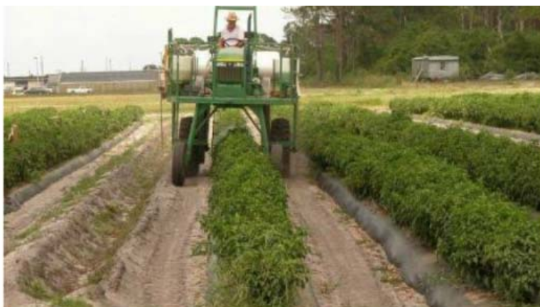
Figure 3. Injection into drip using a 12 V pump and bladder tank
